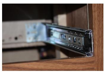
to keep them from opening during travel instead of using on the self-closing type of full extension slides. I didn't think that the spring holding the drawer closed would be strong enough for a drawer full of pots, and other heavy stuff. I looked on line and found the thumb locks I was looking for at:
