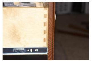
of the old drawers. The screws were removed and the old fronts mounted to the front of the new drawers. Some measuring had to be done to get the old drawer fronts in the correct position to match the location of the original drawers. Once this was done, the drawers were mated to the old drawer fronts. This eliminated having to fabricate new drawer fronts and try to match the stain. Also, new holes were drilled to allow the use of the thumb locks to keep the drawers from opening
