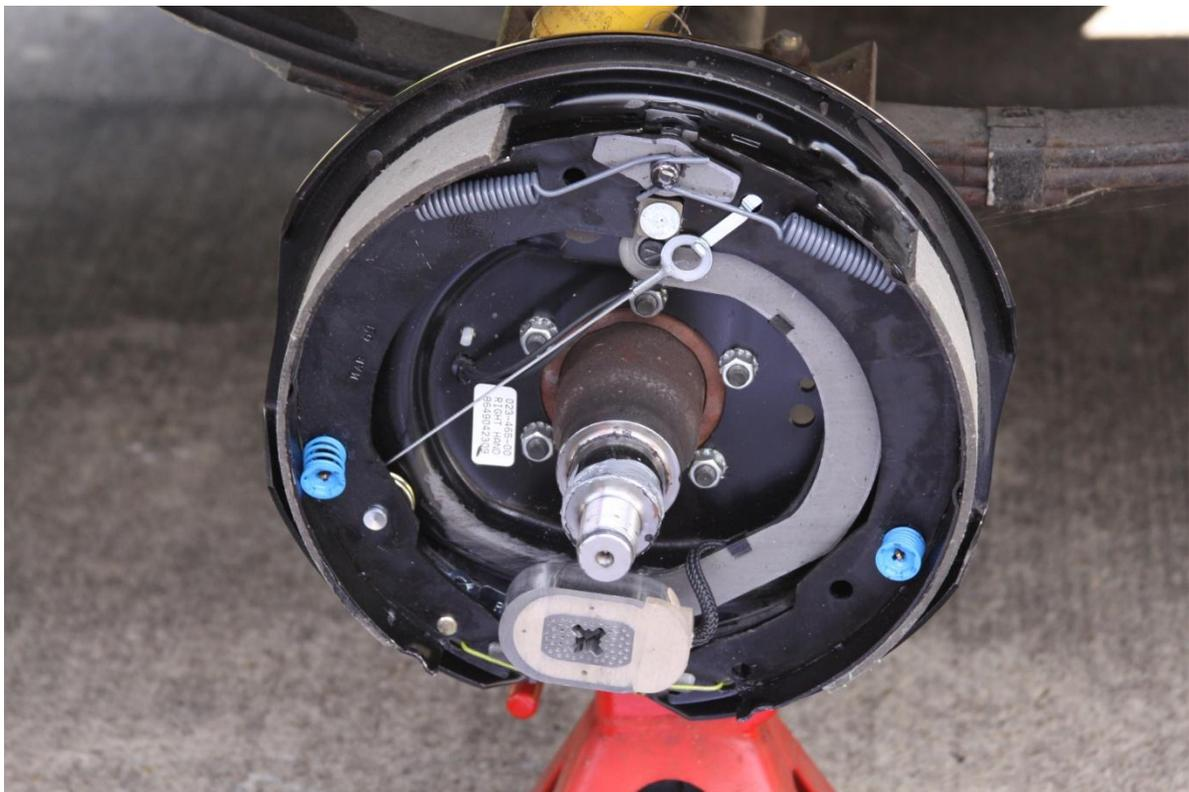
7. The picture above is the new brake assembly mounted on the axle. Now we need to connect the wiring to the trailer. I suggest highly that you use one of two methods. The first is to use marine quality butt connectors that have a heat shrinking material that is heated to shrink around the wire to form a weather tight seal. The second method is to solder the wires together and use heat shrink tubing. Just remember to put the heat shrink tubing on the wires before soldering them together.
