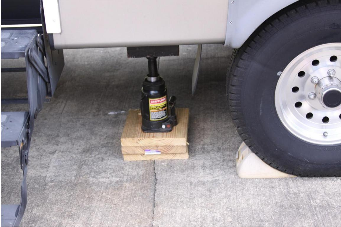
The picture above shows the jack, shoring, and the block between the jack and the frame of the trailer. The picture below shows the trailer on the jack stands with the wheels removed.
