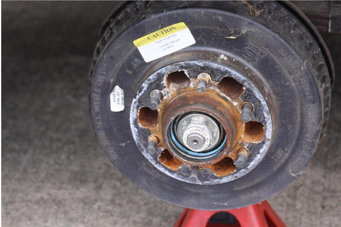
4. Once you have the drum off of the axle, you will see the brake backing plate and shoes and other parts. I suggest at this point in time to reach behind the brake backing plate and cut the wires powering the brake as close to the where they are joined. The connector will be different on all of the trailers but I suggest you cut the wires on the trailer side of the connection.
