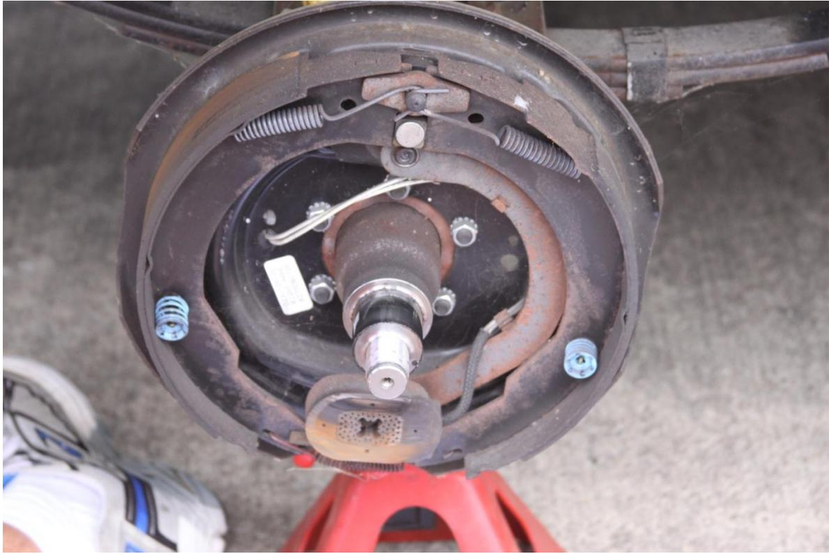
6. Install the new brake assembly on the studs sticking out of the axle and run the nuts down about hand tight. Using a torque wrench, tighten each nut (in a star pattern) to 50 foot pounds.
